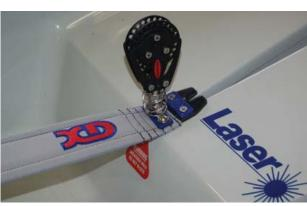
Fit new XD hiking strap and ratchet block using the spring and shackle provided.
