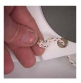
Remove the existing downhaul rope supplied in rudder assembly.
