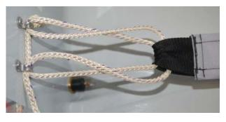
9 The rope tail is then passed through the starboard eye so that the end of the V12 can be pulled from the side of the boat.
