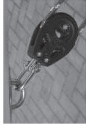
3. Take one of the smaller single vang/kicker blocks and using the shackle provided, attach it to the plate positioned on the lower surface of the boom. (Near the front end).
