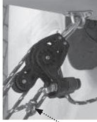
2. Take the short (primary) vang/kicker control line and attach one end to the becket/fiddle on the large double vang/kicker block with cleat using a bowline.
