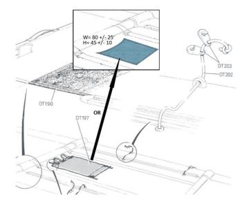
The Satchel DT197 can be replaced with a pocket sewn to the trampoline.
