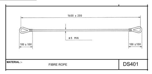
Minimum diameter of the jib strop is reduced to 5mm.
