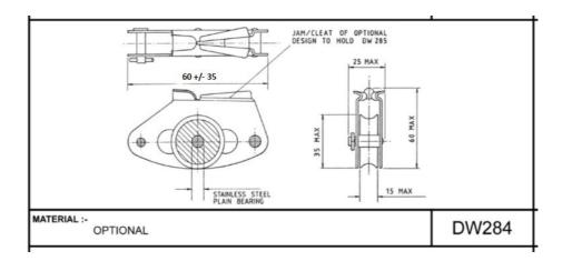
The overall length of DW284 has been adjusted such that the maximum length is 95mm.
