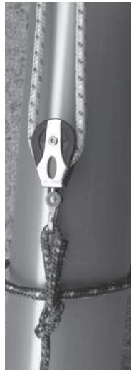
**10.** Insert the standing rigging hound into the track on the front face of the mast as shown. Ensure that the forestay, trapeze wires and shrouds are not tangled. (figure 23)
