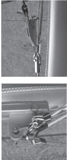
**11.** Attach jib halyard and extension as shown. (figure 24)
